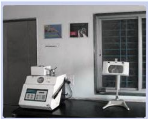
Rockwell Superficial Hardness Tester ( Model : TSM Fine ) having a Rockwell load range of 60, 100 150 kg And Superficial load range of 15, 30, 45 kg.
