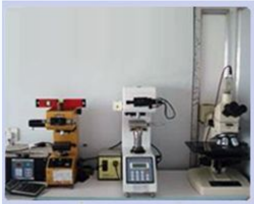
Micro Hardness Tester of Matsuzawa Seiki Co. Ltd., Japan Having a load range of 10, 25, 50, 100, 200, 300, 500, 1000 gms (dial switching) with 100, 400, 1000 x magnification.
